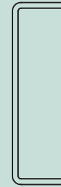
Product SB38x1.2mm G250 Strong Back Channel Lengths Available 3.0m Bundle Qty 20 lengths
